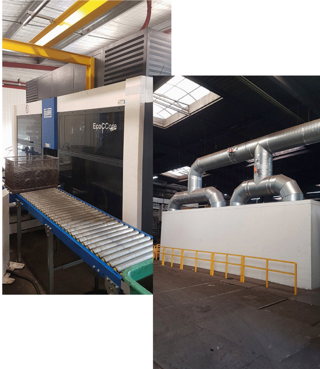
Another important investment concerns a welding cabin for the bogies for better smoke treatment, better ergonomic and working conditions in the workshop.
