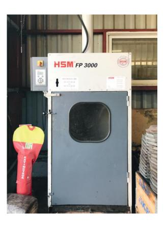
The workshops proceeded for the replacement of plastic containers by the installation of a metal drum press whose main environmental objectives are to:
