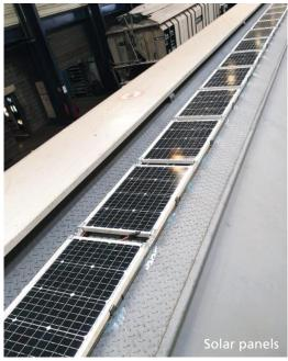
The energy required to operate the onboard systems is provided by solar panels on the railcar's body.
