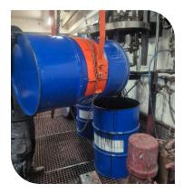
As part of a programme to prevent risks associated with manual handling, a drum turner has been installed to facilitate drum handling during the emptying of paint drum bottoms, to reduce the muscular effort required of the operator during this manual operation and to relieve back strain.
